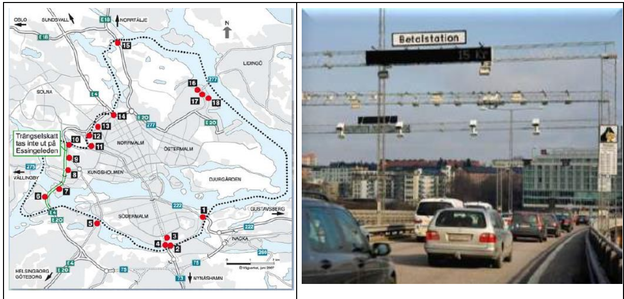
Figure 8.3: Stockholm Scheme Boundary and Example Detection Infrastructure Source: Sweden National Roads Authority
